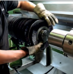
Several segments can be clipped to on one brush holder
