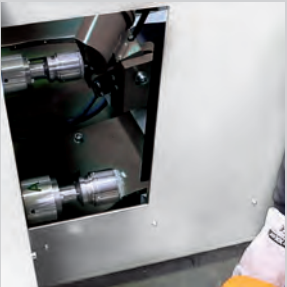
After the trimming process, the engine stops and the door opens automatically
