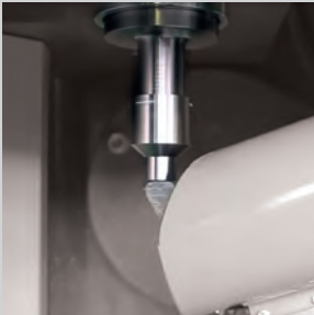
Start of trimming and parallel inserting of the next brush
