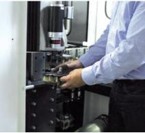
The double sided EdgeRacer<sup>®</sup> is the perfect solution for strongly formed components and precision double sided edge rounding and deburring. This is the first machine of its kind worldwide in series production offering double-sided deburring with reproducible results even on 3D processing. The setting of the brushes above and below the components can be individually adjusted for ensuring optimal results.
